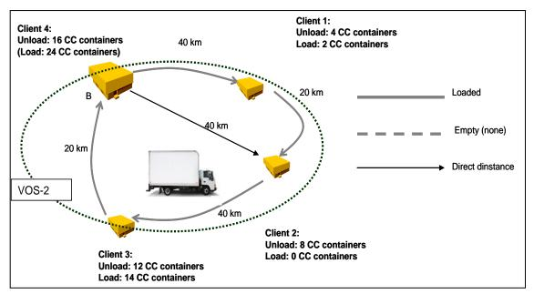
Figure 5.4 Combination of loading and unloading within a single VOS
