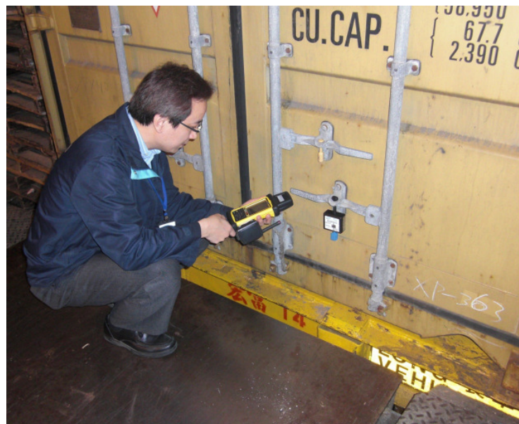
Fig. 42: Reading of container RFID tag and eSeal data using the CHINOS handheld RFID reader
